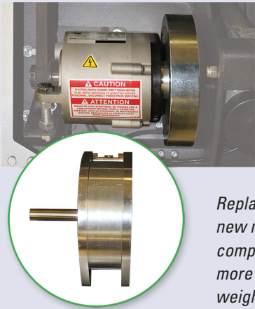
OEM design originally included catalog motor with adapted mounting and added flywheel.
